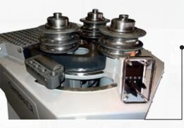
**SB3S-XXX** features hydraulically operated guide rolls that are journaled together with the swing arms of the main bending rolls and automatically follow the adjustment of the lower rolls. The guide rolls are adjustable in&out of the machine frame and around their axis of rotation. For added capabilities, the guide rolls can also be optionally equipped with hydraulically powered traverse axis for fine adjustments in the plane of rolling.
