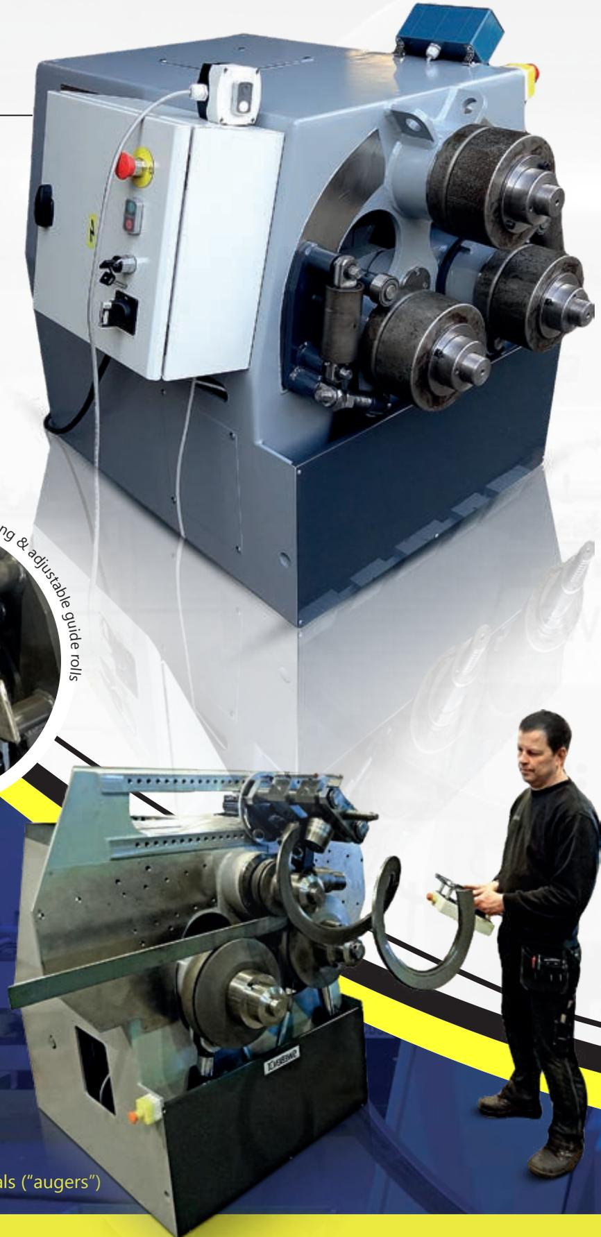
SB3S (Section Bending 3 roll Special) series offers thirteen different models ranging from 7 to 18,000 cm<sup>3</sup> (0.4 to 1100 in<sup>3</sup>). These machines are extremely sturdy in design and have more power compared to any other Section Bending machine on the market. These machines feature hydraulically operated guide rolls.
